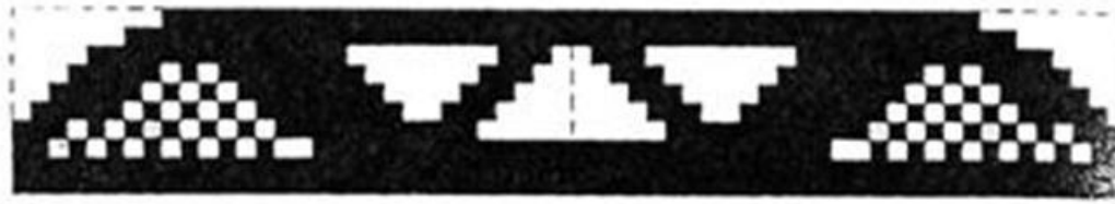
The checkerboard pattern in simply supported beam example [Sigmund and Petersson, 1998]
